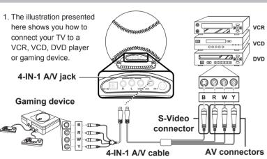
2. The cables are color-coded (black, red, white, and yellow). Connect each color-coded cable to the appropriate connector on your device.
